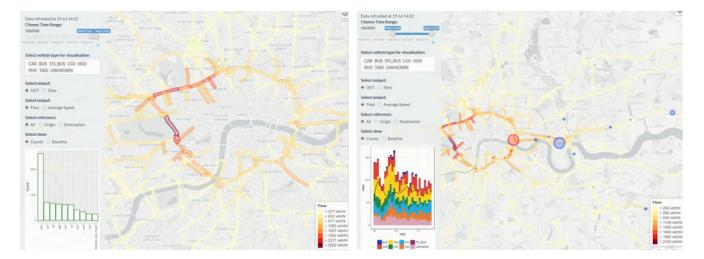
The route monitoring view shows a segmented view of London, broken down into 1 km sections. In this mode, RODAT displays the relative usage of each segment as vehicles complete their journey towards Central London.
